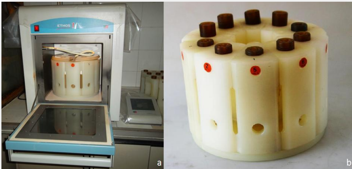
Figura 5.11 – (a) sistema a microonde Milestone ETHOS1. (b) Sistema Milestone® HPR-1000/10S High Pressure.
