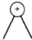
Figure 1.1 Beginning of the creation of a random program tree, with the function + as initial node and two arguments chosen as roots of the tree.
