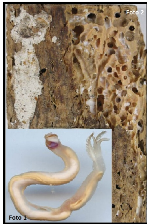
Picture 4.3 Foto 1. T.Naualis; Foto 2. Heavily damaged the wooden structure due to the activities of T.Naualis
