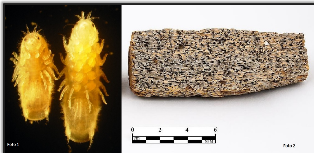
Picture 4.6 (foto1) Gribble Limnoria lignorum ; (foto2) The degradation of wood material caused by the colonization of Gribble Limnoria lignorum
