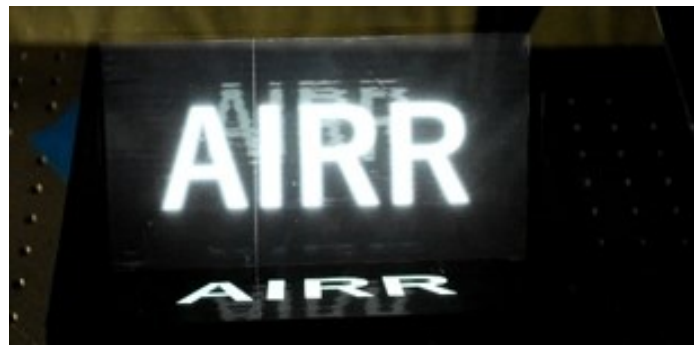
Figura 2.5. Immagine aerea ottenuta attraverso l'AIRR (Terashima, Y., Suyama, S. & Yamamoto, H., Aerial depth-fused 3D image formed with aerial imaging by retro-reflection (AIRR) , Opt Rev 26, pp. 179–186, ( https://doi.org/10.1007/s10043-018-0473-9 ), 2019)
