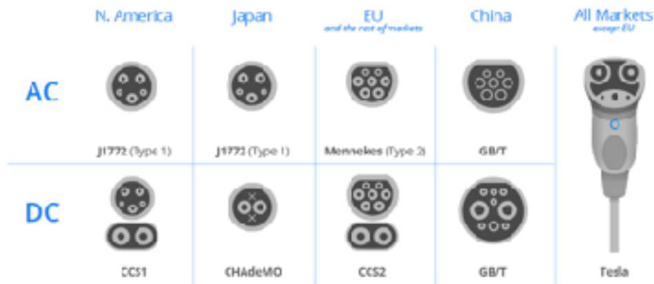
Figure 3: DC fast charging stations' connector types for EV charging around the world
