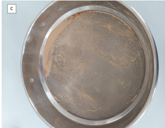
Figure 3. Cabasite 200 mesh retained in the sieve (A mesh 1mm; B mesh 0.5 mm; C mesh 0.15 mm).
