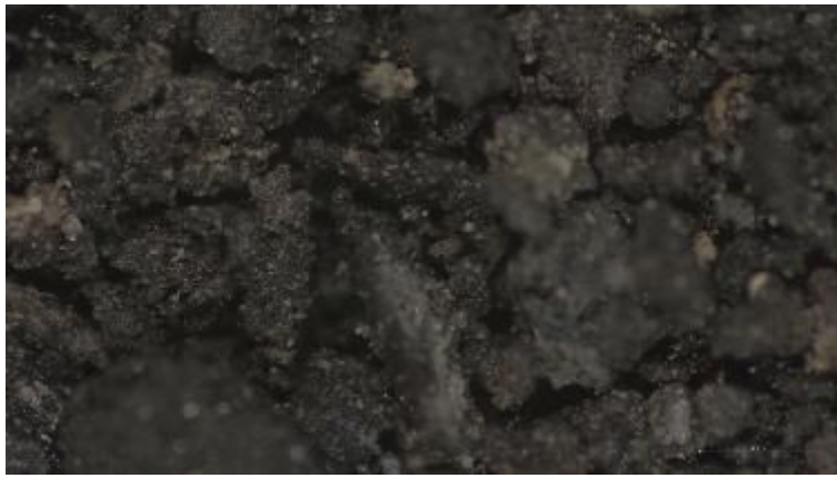
Figure 42. Microscopic picture of black powder, sample G_7 6,3x.
