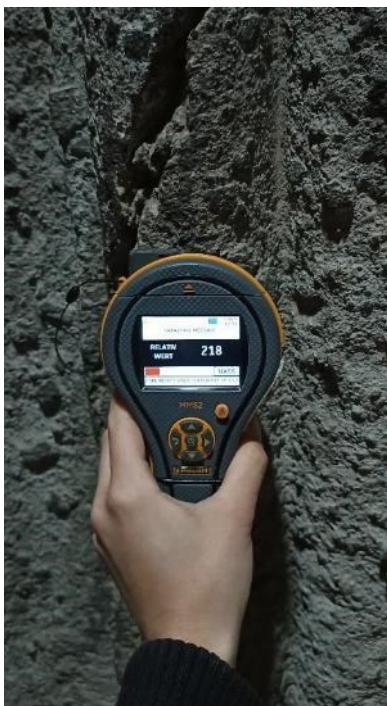
Figure 7. Application of Protimeter MMS2 in "Pinless Moisture Meter" mode.
