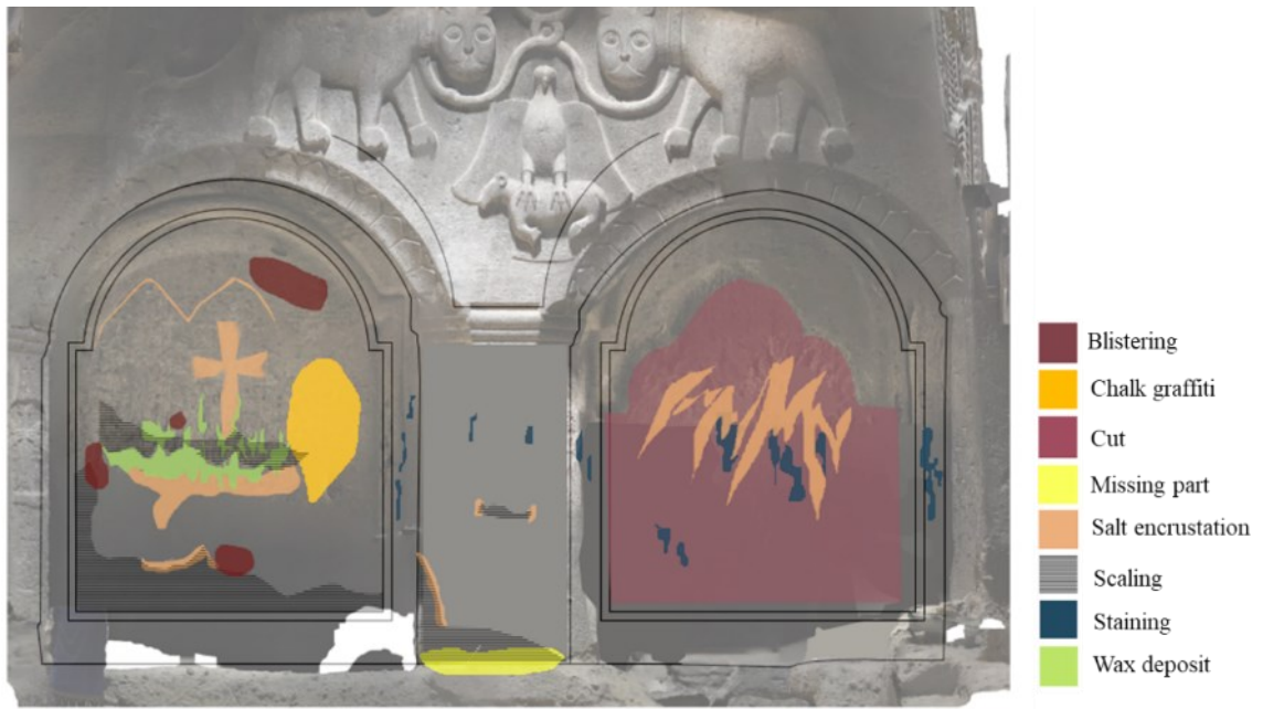
Figure 22. Degradation map of the northern wall of the Proshian family room.
