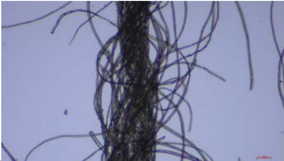
SAV_R 4x: As for the sample L_PET, low magnifications (4x) allow the observation of the twisting of the single fiber that, when intertwined together, form the final yarn.
