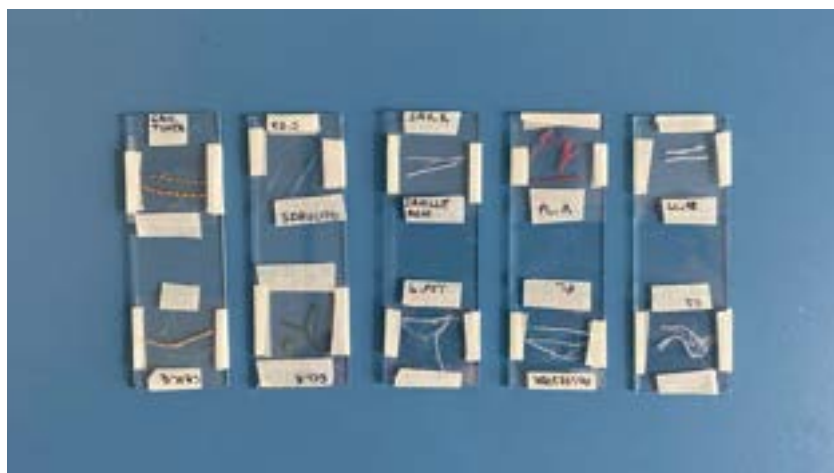
Figure XX: samples prepared on the glass slides for the analysis under Optical Microscope
