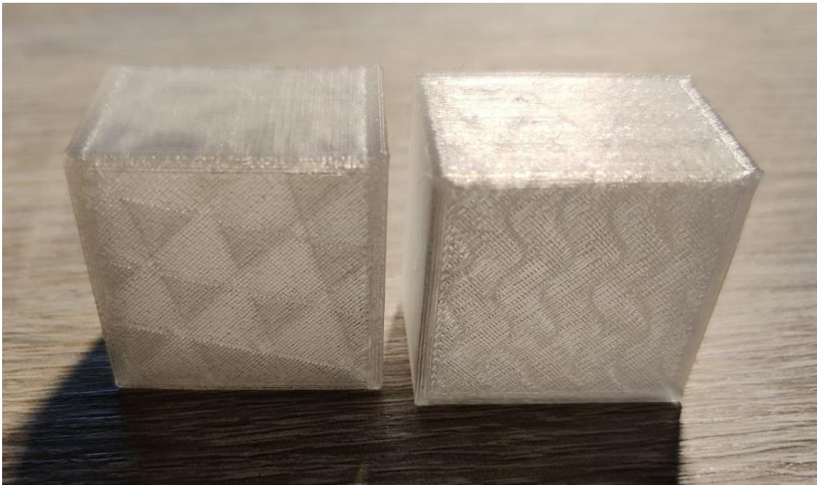
Figure 35. two objects printed in clear PETG, their infill patterns (left: 10% cubic, right: 15% gyroid) are visible through their surface.
