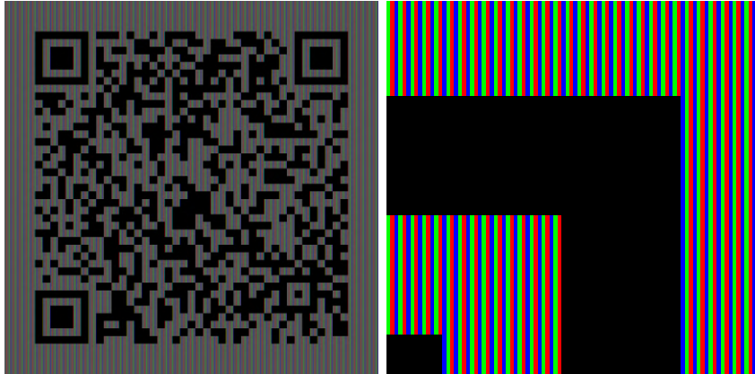
Figure 15: Resulting image of the LCD sampling
