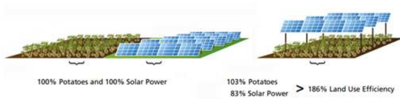
Figure 3.1: Potato growing increased land-use efficiency on the Heggelbach site to 186% (Agrivoltaics a Guideline for Germany, 2022)
