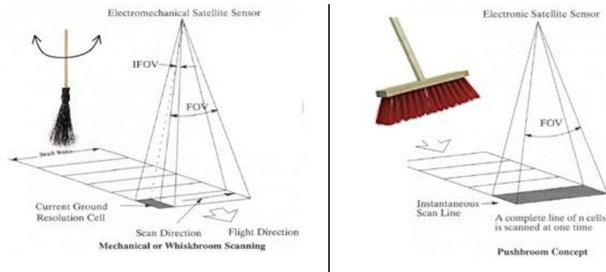
Figure 2.2. Left: basic principle of Whiskbroom scanning. Right: Pushbroom scanning.
