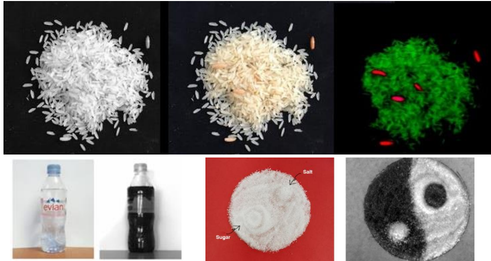
Figure 1.1. Top: Same scene as grayscale image, color image and processed hyperspectral image. Bottom: bottle of water and sugar and salt seen in the visible spectrum and in the short-wave infrared spectrum.
