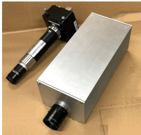
Figure 3.7. The two hyperspectral system, both comprehensive of camera, prism and lens: Vis-NIR (left) and SWIR (right).
