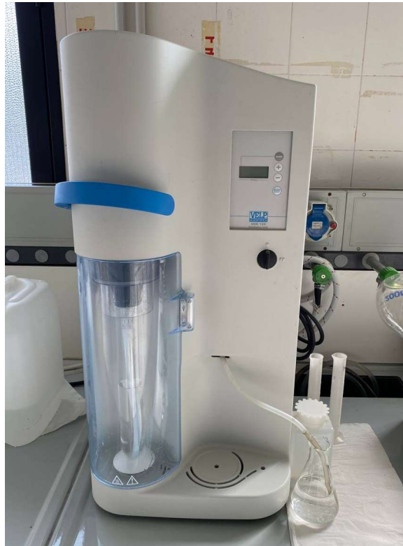
Figure 10 Distiller used for the TKN analysis.
