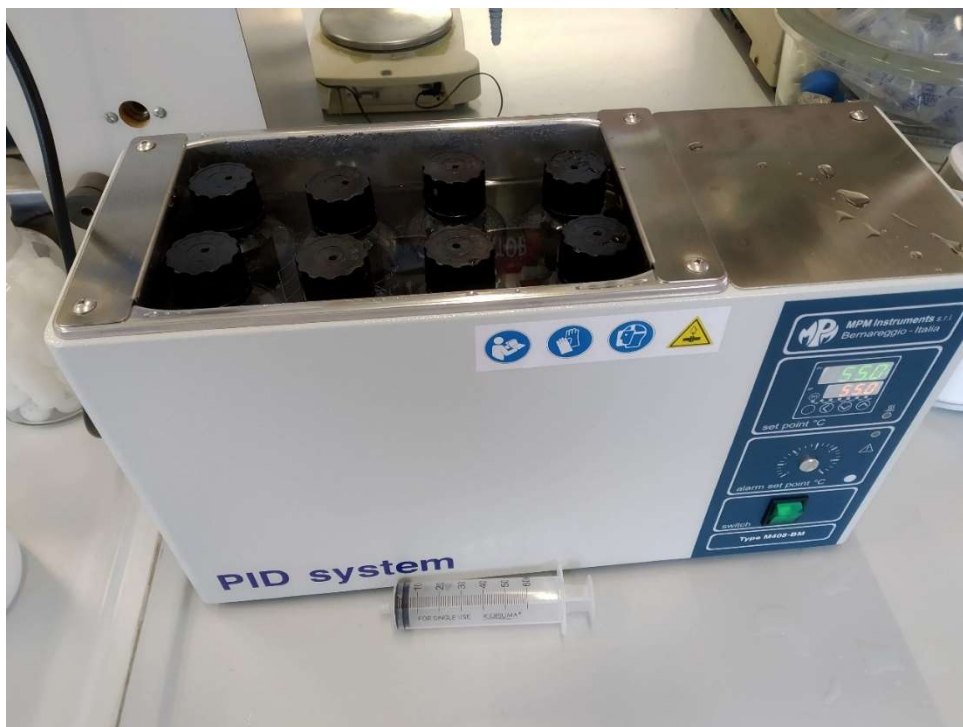
Figure 5 Thermostatic bath used to perform the thermophilic fermentation.
