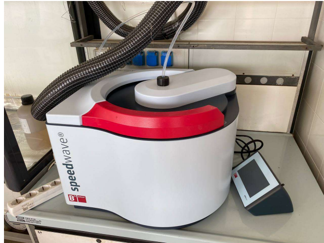
Figure 7 Mineralizer used for the digestion of the dried sludge.
