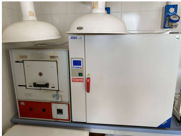
Figure 9 Oven and muffle used to dehydrate/incinerate wet sludge.
