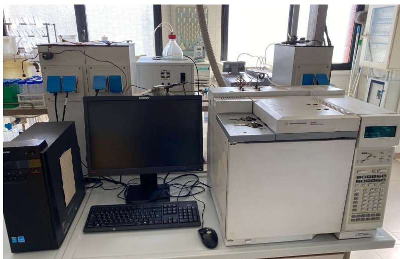
Figure 6 Gas chromatograph used for SCFAs determination.
