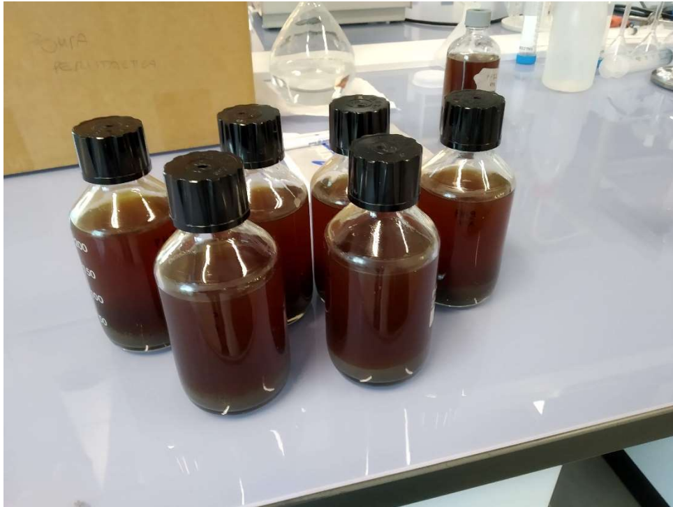
Figure 4 Preparation of the bottles used to perform the acidogenic fermentation after pretreatment of the sludge.
