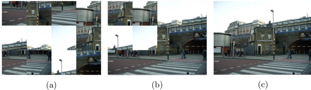
Fig. 19: Example of image reassembling with tile of size 168x168, (a) starting point with all tiles shuffled, (b) the result after extracting compatibility and using Relaxation labeling. (c) original image, the goal.
