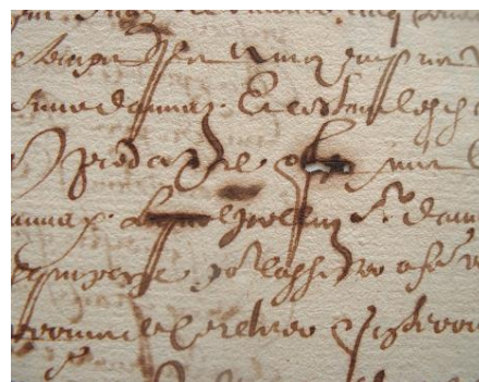
Fig. 14 Degradation in a paper manuscript due to iron-gall inks induced reactions. Adapted from Gimat A. et al, 2016
