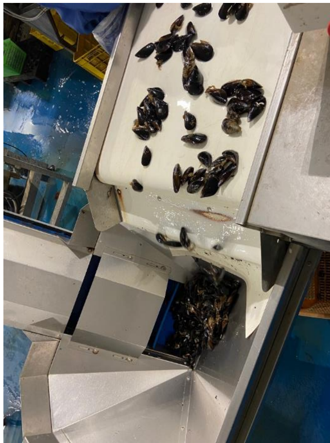
Figure 15 - Conveyor belt for mussels in the Chioggia depuration plant, photo from the visit.
