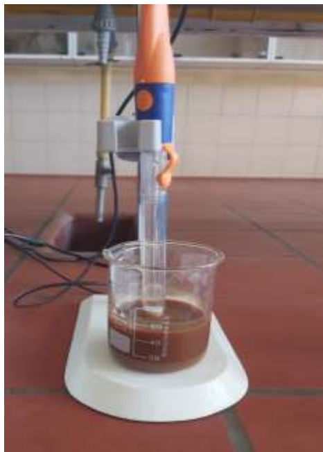
Figure 20: controlling pH after adding \text{NH}_3
