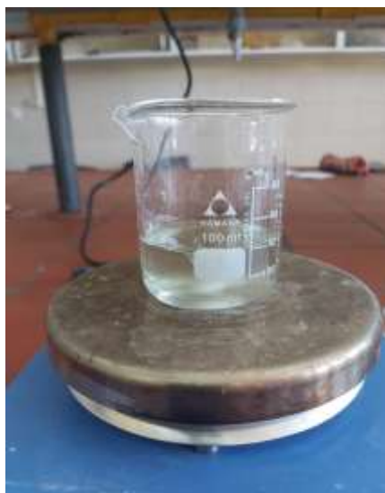
Figure 15: After adding ascorbic acid pH reached to 1.12
