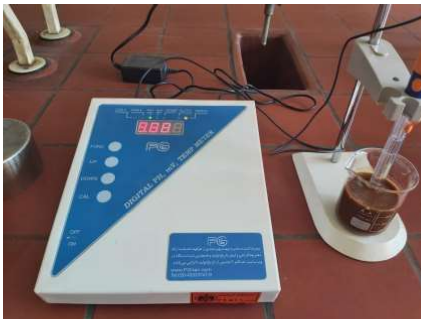
Figure 21: By adding \text{NH}_3 , I adjusted the pH from PH=1.7 to pH=10
