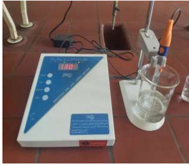
Figure 16: after adding urea pH reached to 1.30
