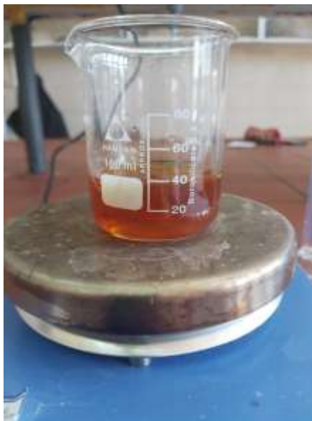
Figure 14: after adding 3 salts. pH reached to 1.7
