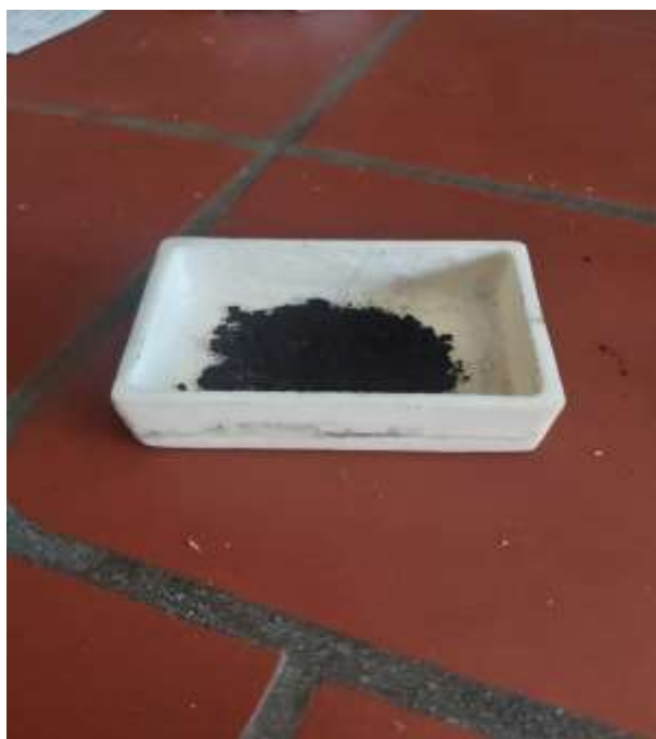
Figure 18: The resulting precipitates after annealing for 500°C for 2 hrs.
