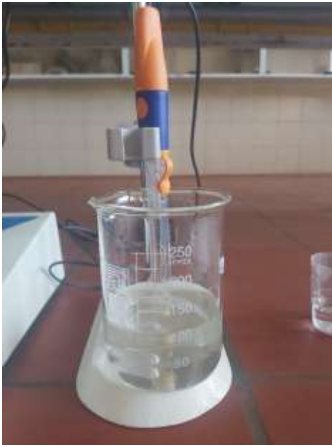
Figure 16: after adding urea pH reached to 1.30
