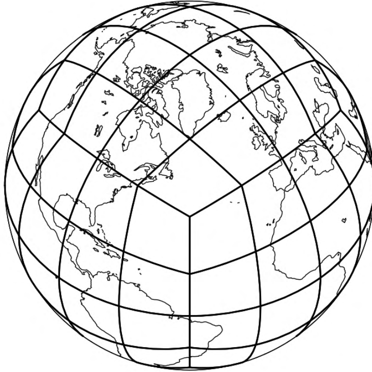
FIGURE 3.2: The cubed-sphere grid geometry with n_e = 4 . Image from (Neale et al., 2012).
