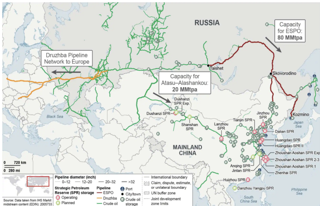
Figure 26: Russian crude oil pipeline and storage system. Source: IHS Markit.
