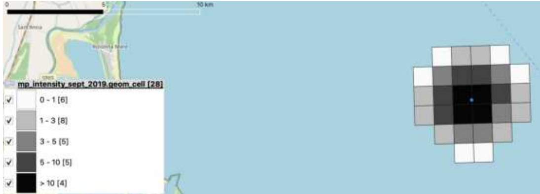
Figure 4.6: Underwater sound propagation in an instant of time of the boat CARLO ALBERTO II which is carrying out a fishing activity.
