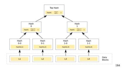
Image 13 shows how 4 different data transactions are validated. Each data block is individually hashed (Hash 0-0; Hash 0-1; Hash 1-0; Hash 1-1), then each couple of hash is hashed and stored into a parent node (Hash 0 and Hash 1), finally the two parent nodes are combined into the final node which provides a timestamp and a nonce which is used to generate the block header. Therefore, Merkle trees provide the hash-based architecture or blockchain which ensures data integrity.
