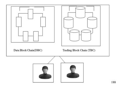
The two blockchains operate in an independent manner, the Data Blockchain (DBC) stores the actual user data and the trading Blockchain (TBC) stores only relevant information which is useful for executing the transaction. Both blockchains exchange information between each other and data authenticity is achieved via cryptographic techniques<sup>189</sup>.
