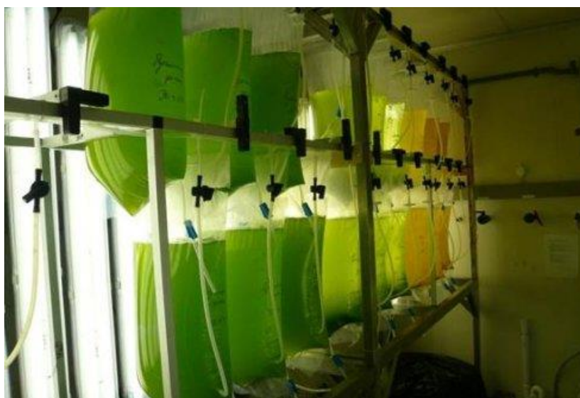
Figura 6 - Bag system (Indoor algae culture system – WUR).
