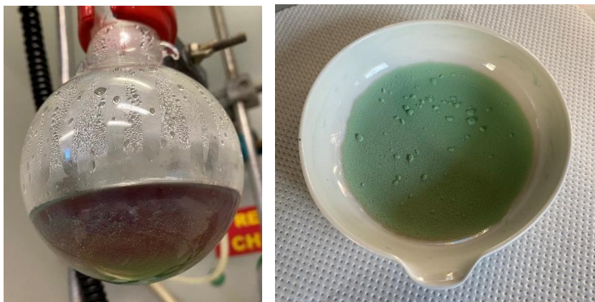
Figure 2.4.1. Pictures of NiCo LDH after 3 hours of reflux (left) and after drying (right).
