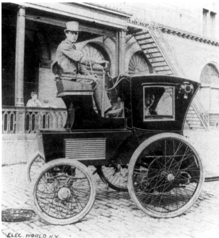
Electric hansom cab produced by the ECWC, 1897, Electric Motor Cab Service in New York City, Electrical World , August 14 th , 1897 29
