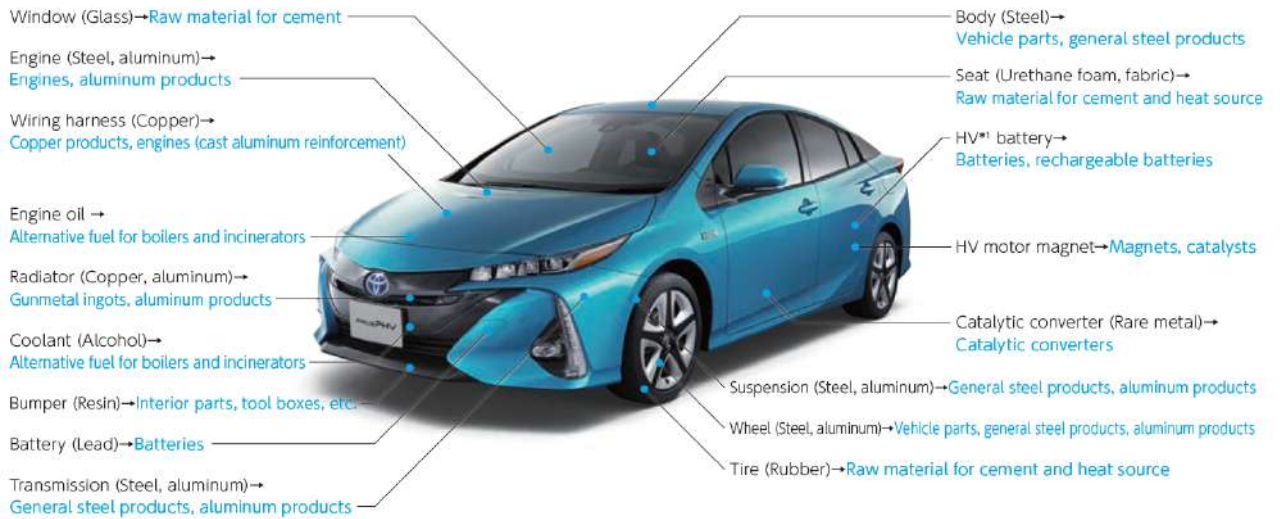
Figure 84: Prius recycling scheme
