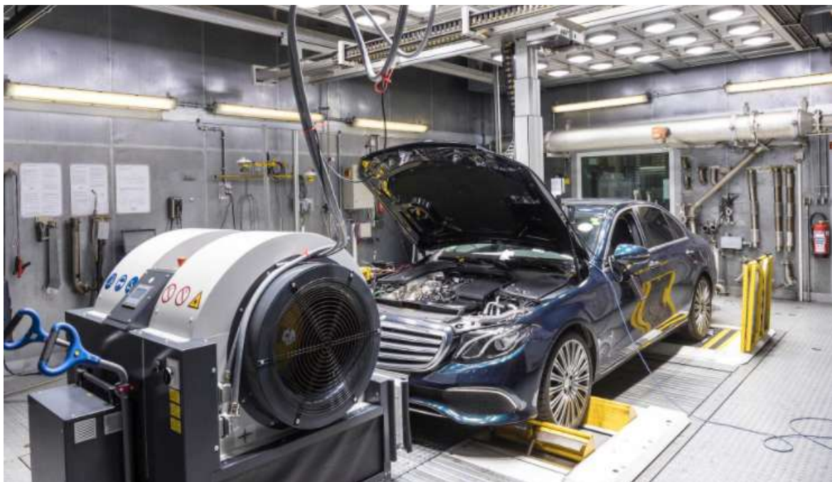
Figure 32: WLTP test in the laboratory
