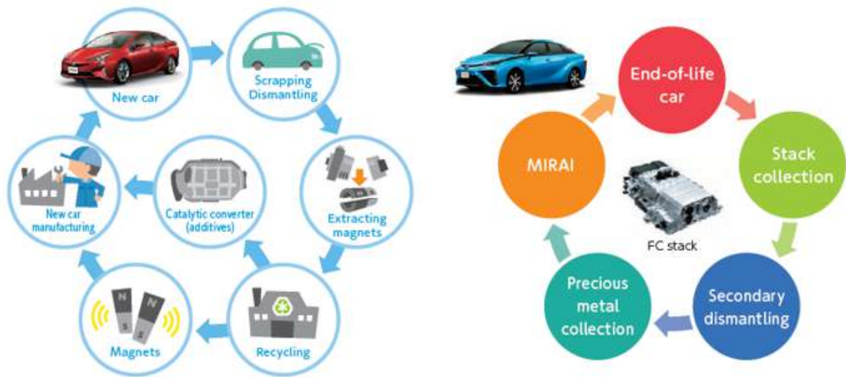
Figure 82: Magnets and Fuel-cell stack Recycling scheme
