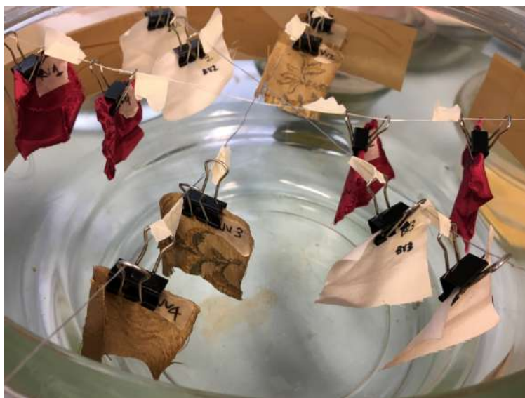
Figure 3: silk samples hanged in the desiccator before exposure to sanitising solution's vapours
