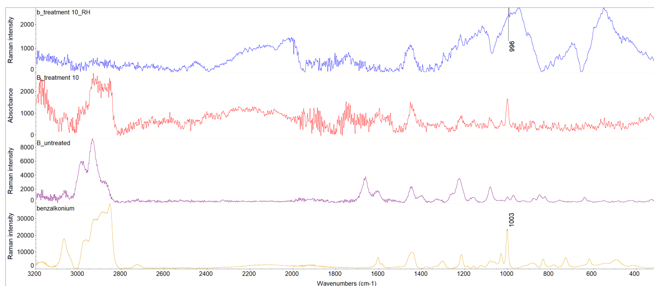
Figure 29: comparison of three white silk Raman spectra (untreated, after treatment 10 and after treatment 11) and Raman spectra of benzalkonium chloride
