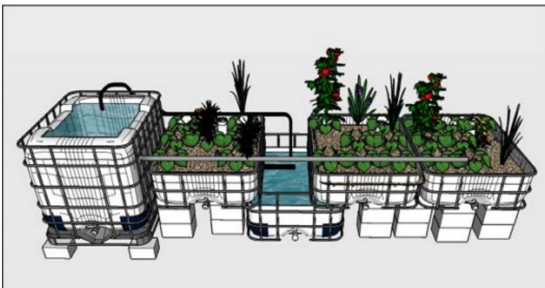
Figure 13: Example of Media bed-system aquaponics Source: Sommeville et. Al 2014
