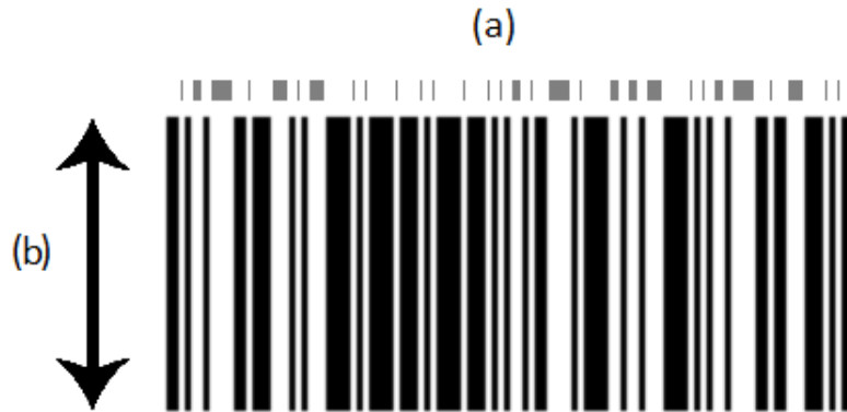
Figure 1: Structure of one-dimensional barcode. (a) shows the variation of the space between the vertical lines. (b) shows how the widths of the vertical lines can change.
