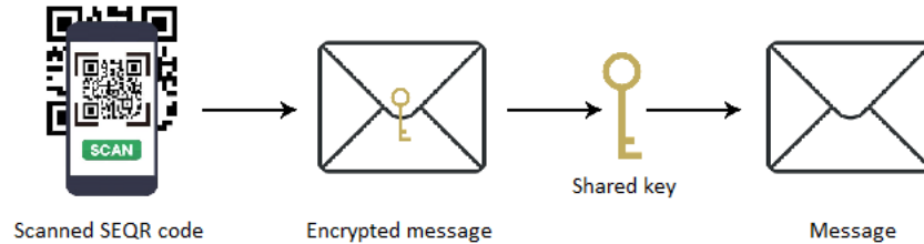
Figure 12: Decryption process for read the content of a SEQR code.
