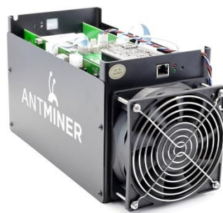
Figure 12: Bitmain Antminer Bitcoin Mining Hardware
